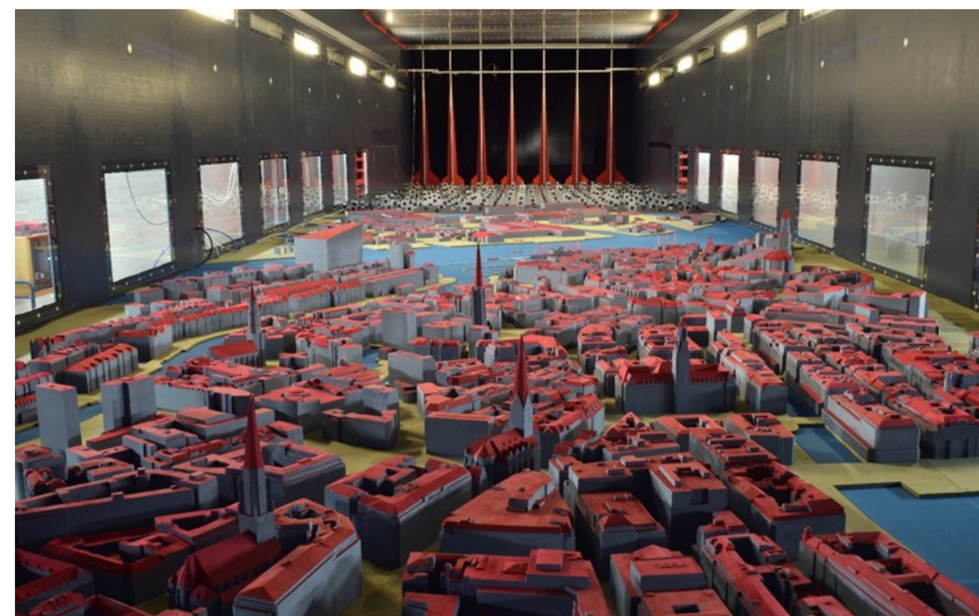
3 Upwind view of the wind tunnel model of Hamburg's city.
