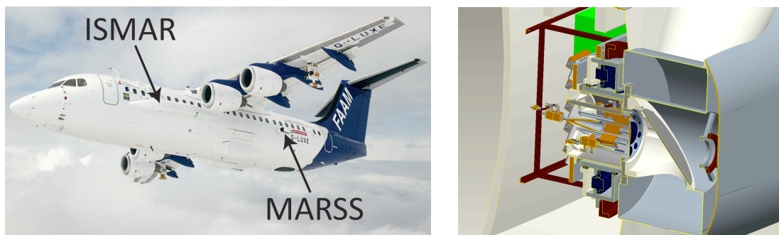
Figure 4.7: Left: The FAAM aircraft with the positions of ISMAR (submillimeter channels) and MARSS (183 GHz and below). Right: A cutaway view of ISMAR mirror, scan drum, and feedhorn cluster.
