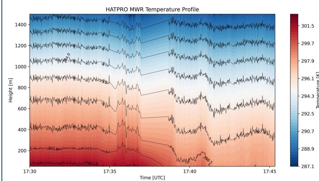
Vertical profile of temperature indicating temperature drops up to heights of 1000 m during cold pool event, corresponding to the **cold** pool depth.
